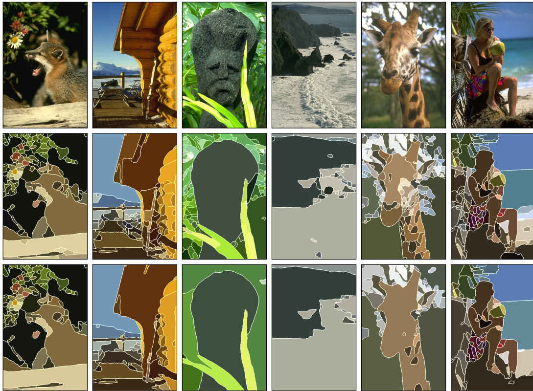
Figure 8.4: Additional segmentation results on the BSDS500 produced by the gPb-mad-esm algorithm using a constant value threshold. From top to bottom: input image, and segmentations corresponding to the optimal dataset scale (ODS) and optimal image scale (OIS). All images are from the test set.
