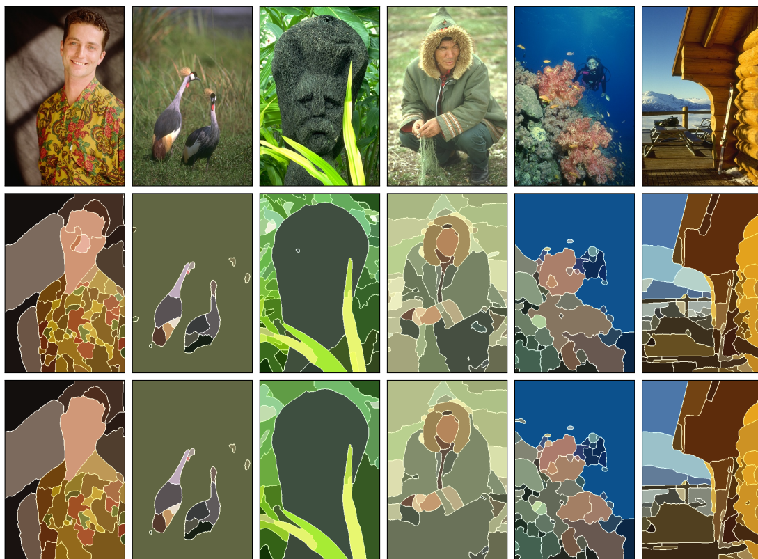
Figure 8.6: Segmentation results on the BSDS500 produced by the gPb-mad-sfm algorithm using a threshold based on region size. From top to bottom: input image, and segmentations corresponding to the optimal dataset scale (ODS) and optimal image scale (OIS). All images are from the test set.
